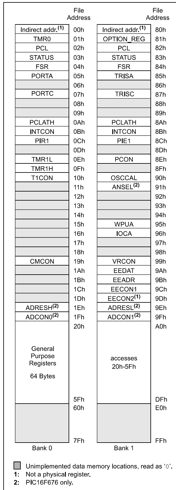
FIGURE 2-2: DATA MEMORY MAP OF THE PIC16F630/676
